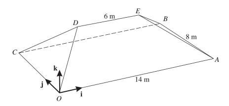
The diagram shows the roof of a house. The base of the roof, *OABC*, is rectangular and horizontal with OA = CB = 14 m and OC = AB = 8 m. The top of the roof *DE* is 5 m above the base and *DE* = 6 m. The sloping edges *OD*, *CD*, *AE* and *BE* are all equal in length.
